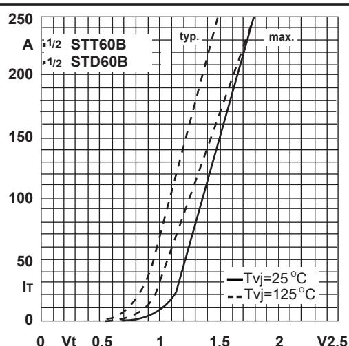
Fig.7 On-state characteristics
